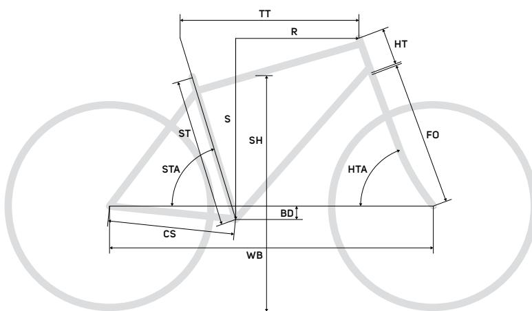
FS = ST frame size = seat tube [mm]   TT top tube [mm]   HT head tube [mm]
