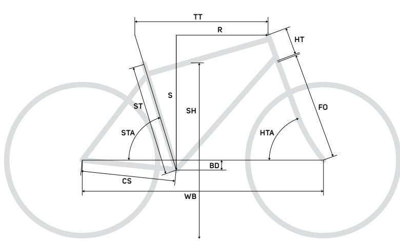
FS = ST frame size = seat tube [mm] TT top tube [mm] HT head tube [mm]
