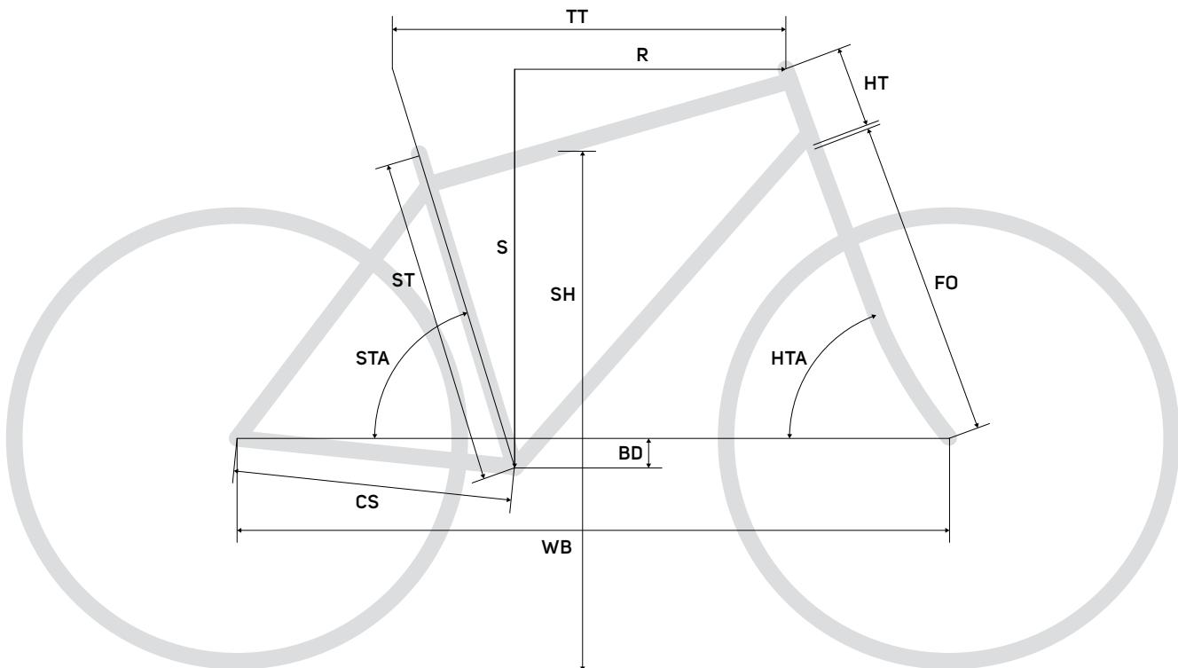
FS = ST frame size = seat tube [mm] TT top tube [mm] HT head tube [mm] HTA head tube angle [°]
